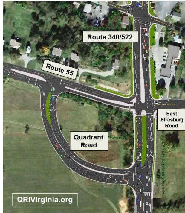
The QRI was chosen for this congested area because it handles more vehicles and offers fewer delays than a conventional four-way signalized intersection. This is achieved by moving left-turns away from the intersection of Route 340/522 and Route 55, and relocating them to the intersections with Quadrant Road. The QRI provides substantially more green-light time for north-south traffic on Route 340/522, which is the dominant pattern at this intersection.
